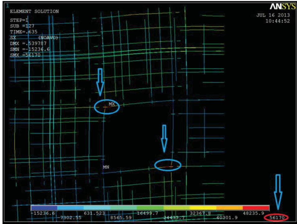
Figure 6.8: First Yielding of Steel Rebars at Opening (14%) Corners, at Load of 76.2 kN
