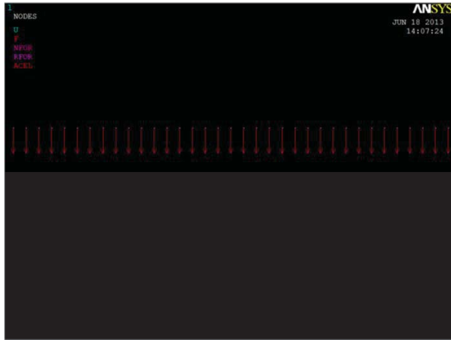
Figure 4.21: Application of Live Load in FE model
