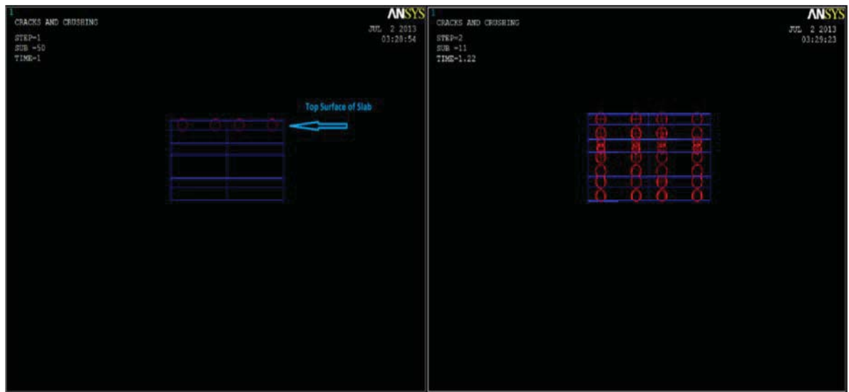
Figure 5.10: Extension of Cracks Inwardly (in depth of slab)
