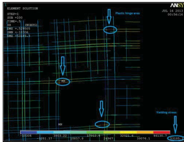
Figure 6.11: Yielding of Steel Rebars at Corner of Opening
